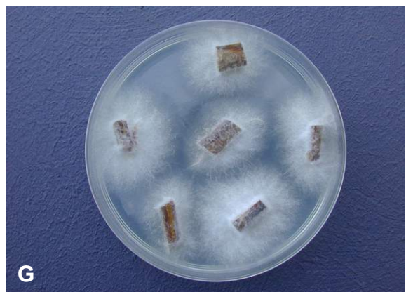
Figure 6. Techniques used to evaluate treatments for the prevention of wound infection: (A) Cutting canes to two-bud spurs on Cabernet Sauvignon vines at Nuriootpa; (B) Applying treatment to wound with a paint brush; (C) Inoculating treated wounds with ascospores of E. lata ; (D) Spurs removed from vines during the following winter; (E) Spurs with bark removed; (F) Cutting chips from either side of the necrotic margin and (G) Cultures of E. lata growing from wood chips.
