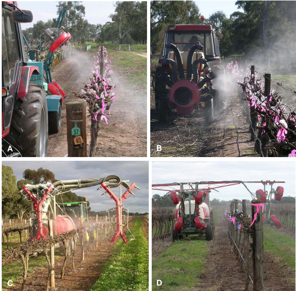
Figure 11. Sprayers used for trials at Nuriootpa Research Centre in 2004 and 2005; (A) SARDI fan sprayer (prototype) and (B) Hardi air-assisted sprayer and Coonawarra in 2007 and 2008; (C) Silvan Turbomiser and (D) Croplands Quantum Mist.
