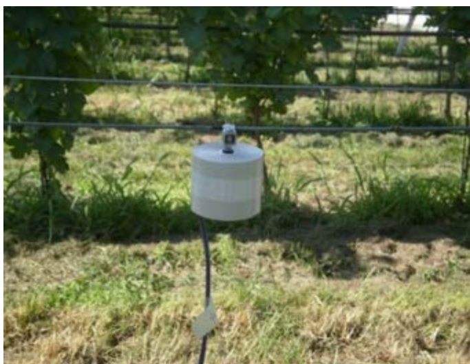
Figure 2: Shaker designed to transfer disruptive noise to longer distances. (Source: Lucchi et. al)
